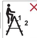
Do not stand on the last two steps of the ladder in A position.
