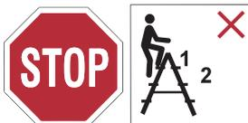
Do not stand on the last two steps of the ladder in A position.
